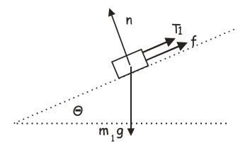
We did not draw in the force down the ramp as it is a component of the weight vector, mg which we did draw. It would not have been wrong to draw it in, however. The forces are: the weight, mg; the normal force, n; the tension in the string  $T_I$ ; and the frictional force, f. The frictional force is directed up the ramp because the block is sliding down the ramp and the force of friction is always opposite to the direction the block is moving.
