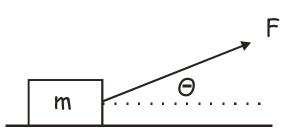
The complication in this problem is that F has a horizontal and vertical component. We draw the FBD. The components are  $F \sin \theta$  and  $F \cos \theta$ .
