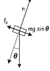
If the block moves at constant velocity, then the net force down the ramp is zero. This means that the kinetic force of friction must equal the force component down the surface of the ramp. First let us find the kinetic force of friction:
