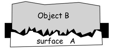
Another cause of friction is deformation of the surface. An object sitting on a surface causes the surface to sag a little. So the object is sort of sitting in a little depression. To make it move, you have to dislodge it from the depression it's in. (This is similar to what the Physics Kahuna experiences with a class on Monday morning, to get the class moving, he must dislodge it from the depression each student is in.)
