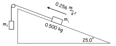
First, we draw the appropriate FBD's. Then we can analyze the forces acting on each block.
