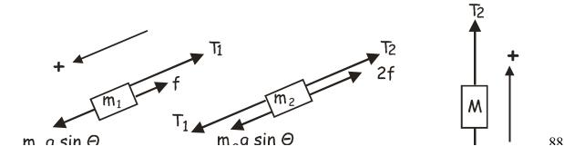
$\sum F = 0$  $m_1g\sin\theta - T_1 - f = 0$ For block 1:  $m_2g\sin\theta + T_1 - T_2 - 2f = 0$ For block 2:  $T_2 - Mg = 0$ For block M:  $m_1g\sin\theta - T_1 - f = 0$ +Add the three equations:
